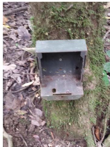
**Figure.2:** Weatherproof metal case for camera trap drilled into a tree, where midpoint of casing is 40cm high.
